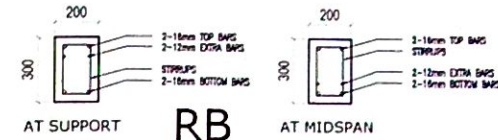
4 BEAM DETAIL SCALE: S 10 1:25m
